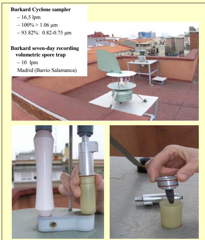
Fig. 1. Hirst-type volumetric trap and Burkard Cyclone samplers. Particles were collected directly into a 1.5 mL Eppendorf vial.
